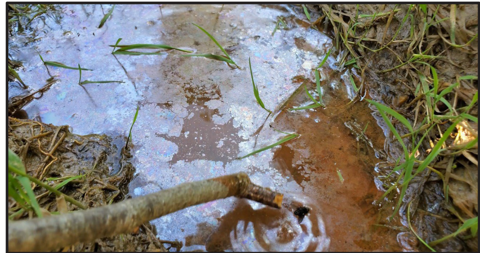
The sheen from iron-oxidizing bacteria remains broken when disturbed with a stick. Try the "stick test" yourself! Photo by Megan Bolcar.
