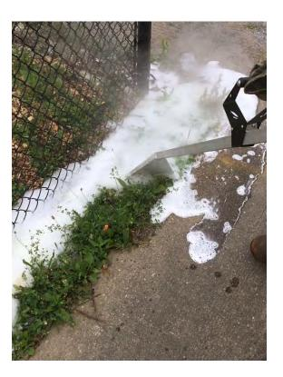
Prior to the introduction of the hot foam equipment, staff were expending significant labor to control vegetation in these spaces, mainly by hand or through a string trimmer or similar equipment. Hand pulling can successfully remove plant root systems, but string trimmers are only able to remove surface vegetation. The use of hot foam can more directly target and cause damage to all parts of a plant, providing longer-lasting control of unwanted vegetation.
