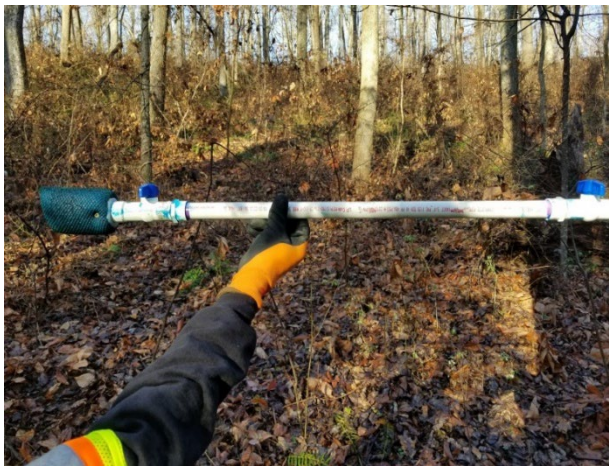
Pictured above (left) is the dauber tool. The sponge tip is on the left and the control valve on the right. Right, is a pesticide applicator carefully applying product to a cut stump. The adjacent ferns are protected from this application by the dauber tool.
